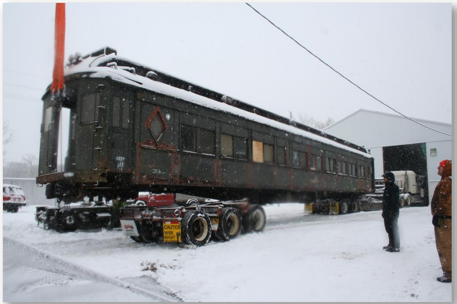
DL&W 3453 gets lifted off of its wheel set and placed on a bogie behind an 18-wheeler. Photo by Dan Morgan
